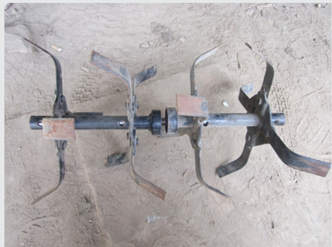
Shaft containing rotary cutters
